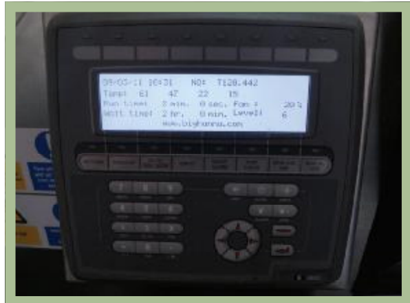
The easy to use control panel. Shows the temperatures on the display for each part of the machine.
